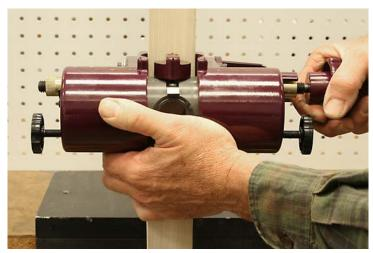
Clamp the HIT-44 to the door with a light pressure, just enough to hold it on the door.
