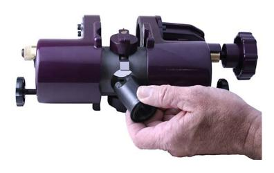
There are three drill guide bushings supplied with the HIT-44 for use when drilling the edge bore, they are held in with a clip. Choose from a 7/8", 1" or the brass guide for use with a multispur bit, they just snap in.
